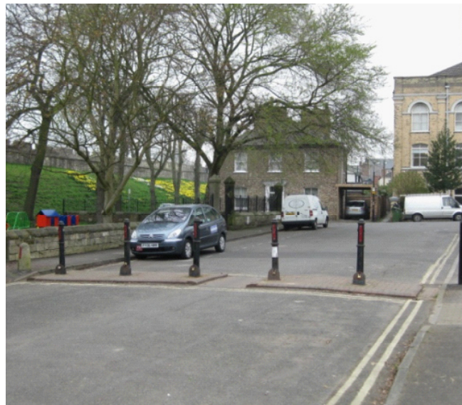
Above: Build-outs provide opportunities for additional cycle parking Below: Road closures which allow cycle access are effective at stopping rat-running whilst promoting cycling permeability
