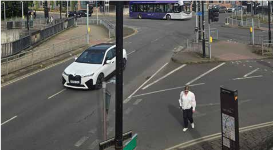
Figure 124 Facilities enabling pedestrian movement should be designed according to how people behave: we recommend designing crossings which accommodate pedestrian desire lines
