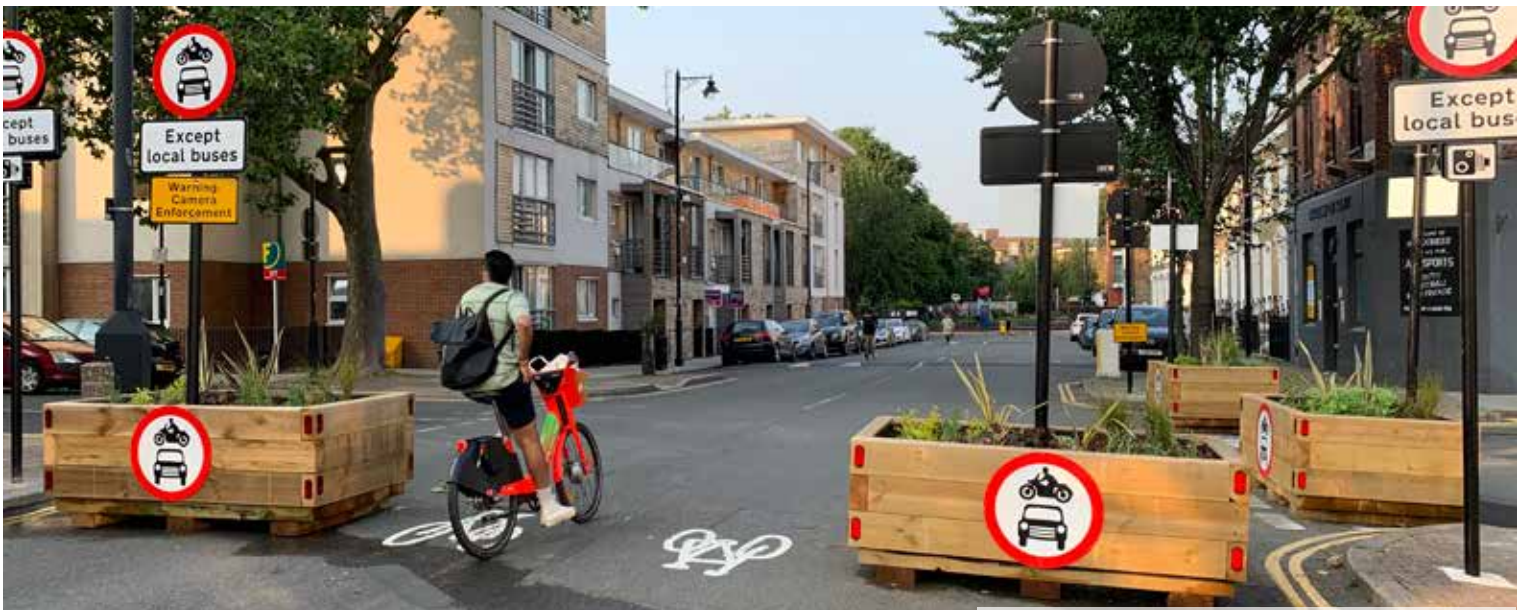
Figure 170 Clean air, low motor traffic and no traffic noise on streets make people feel safe and relaxed. A modal filter prioritising walking, wheeling, cycling and bus travel along Prebend Street in Islington (London)
