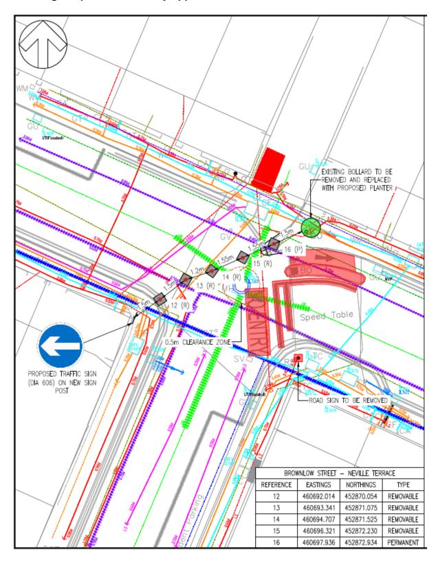
Brownlow Street/Neville Street permanent closure point – proposed design showing the position of utility apparatus under the road surface
