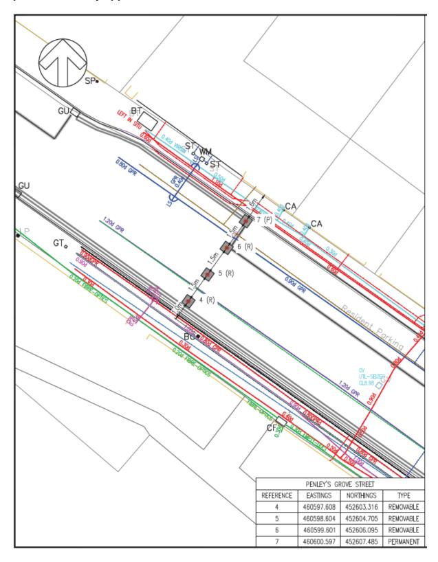
Penley's Grove permanent closure point – proposed design showing the position of utility apparatus under the road surface
