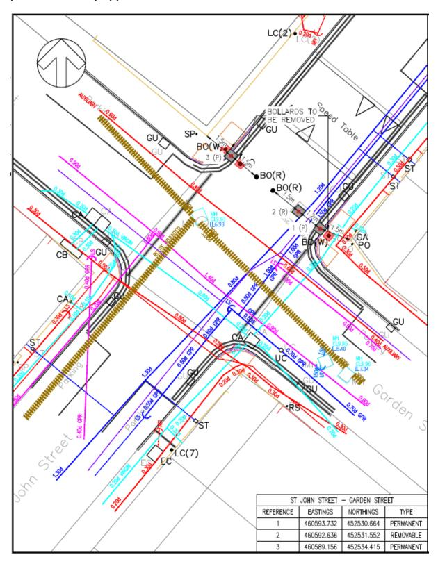
St John's Crescent permanent closure point – proposed design showing the position of utility apparatus under the road surface
