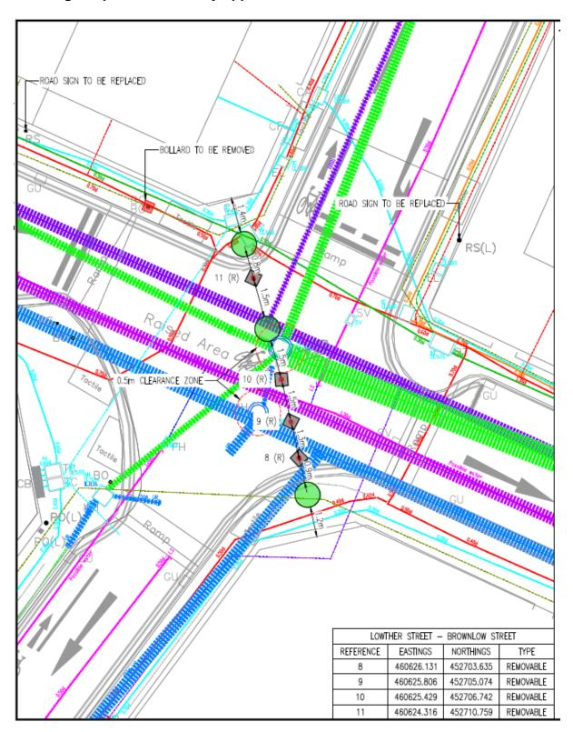
Lowther Street/Brownlow Street permanent closure point – proposed design showing the position of utility apparatus under the road surface
